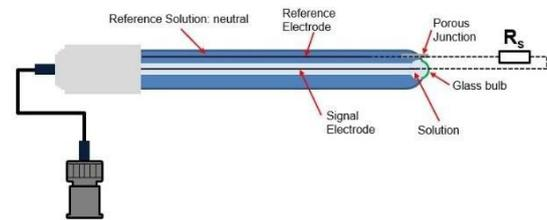
A pH sensor measures the acidity or alkalinity (pH) of a solution by detecting the concentration of hydrogen ions using a glass electrode, a reference electrode, and a pH meter, displaying the pH value on a scale of 0 to 14.
