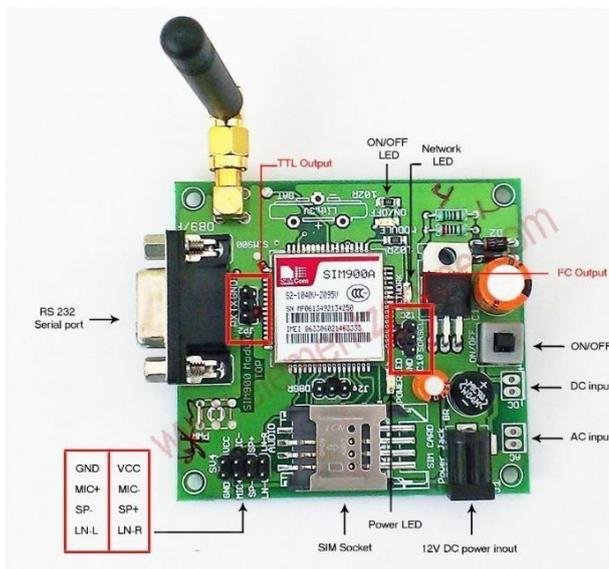
**Data Communication:** The Arduino uno connects to a GSM module, typically via UART communication. The GSM module has a SIM card for cellular data access.
