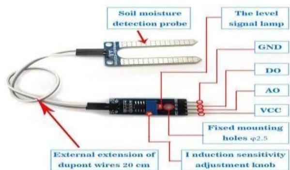
Soil moisture sensor using a measuring moisture level and get moisture level like a Dry or wet, normal. Dry: (520 430], Wet:
