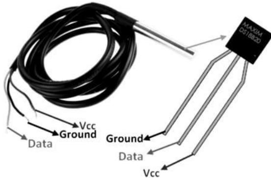
As this is a 1-wire digital temperature sensor, it needs only the data pin and GND pin to interface with the Arduino or microcontroller. The temperature sensing of the sensor ranges from -55°C to +125°C with an accuracy of ±5°C. It is the best temperature sensor to measure the temperature value at multiple points and requires only one data/digital pin of the Arduino or microcontroller unit to transfer the data.
