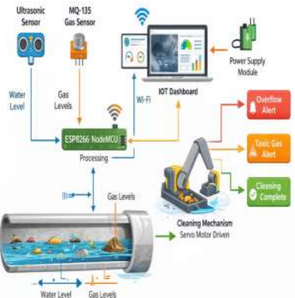
Block Diagram of IoT-Based Smart Drainage Monitoring and Cleaning System
