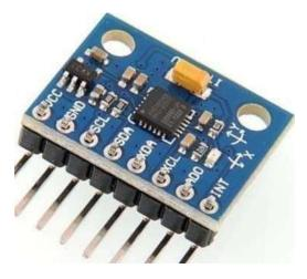
Fig. 3 Accelerometer and gyroscope
