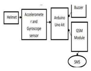
Fig. 1 System architecture.
