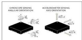
Fig. 4 axis and angular orientation
