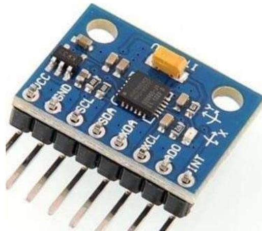
Fig. 3 Accelerometer and gyroscope
