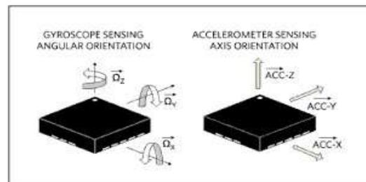
Fig. 4 axis and angular orientation
