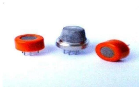
The ALCOHOL Sensor (MQ2) module may be used to detect gas leaks (home and industry). H<sub>2</sub>, LPG, CH<sub>4</sub>, CO, alcohol, smoke, and propylene may all be detected with this device. Its great sensitivity and quick reaction time allow for immediate measurement. A potentiometer allows you to fine-tune the sensor's sensitivity.
