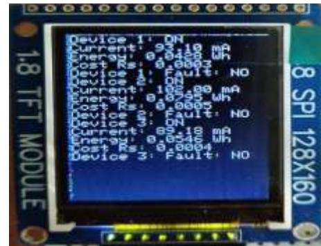
Fig -4(b): Results displayed in TFT display
