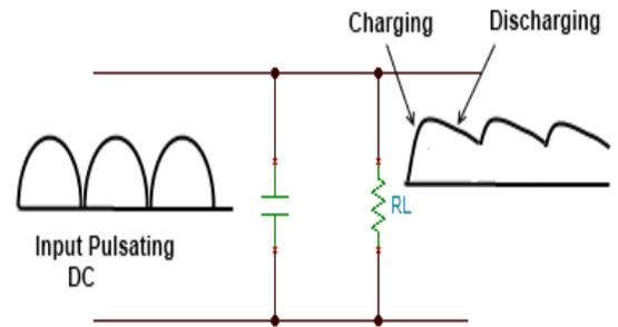
Fig 3.1.3 Filter Circuit
