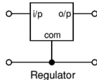
Fig 3.1.4.1 Regulator Circuit
