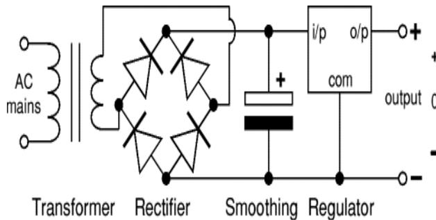
Fig 3.1.4.2 Power Supply Circuit
