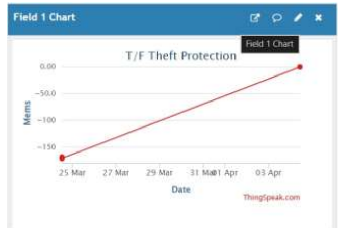
Fig. 5. Field 1 — ADXL345 Accelerometer X-axis Reading (Theft/Movement Detection)
