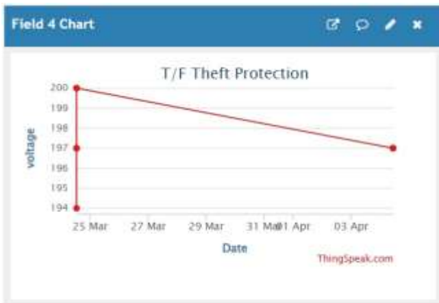
Fig. 8. Field 4 — Supply Voltage (V) Measured by Voltage Divider Network
