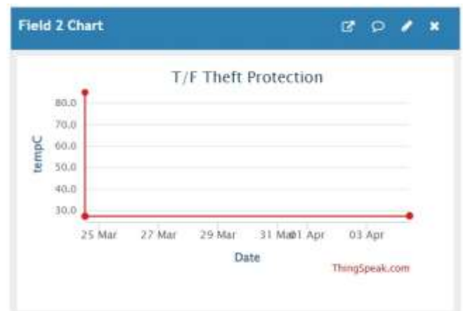
Fig. 6. Field 2 — Transformer Oil Temperature (°C) with Simulated Thermal Fault
