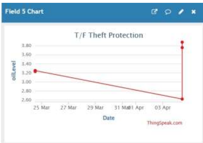
Fig. 9. Field 5 — Oil Level Distance (cm) Measured by HC-SR04 Ultrasonic Sensor
