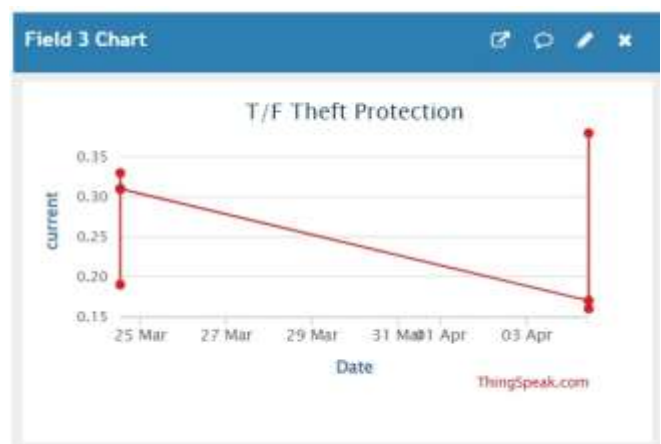
Fig. 7. Field 3 — Load Current (A) Measured by ACS712 Sensor
