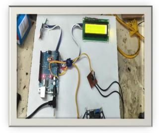
application or web page using the think speak IoT platform. So that the solar panel can be monitored remotely.
