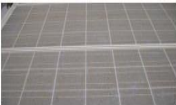
Fig. 3: Solar module covered by heavy layer due to dust accumulation before cleaning
