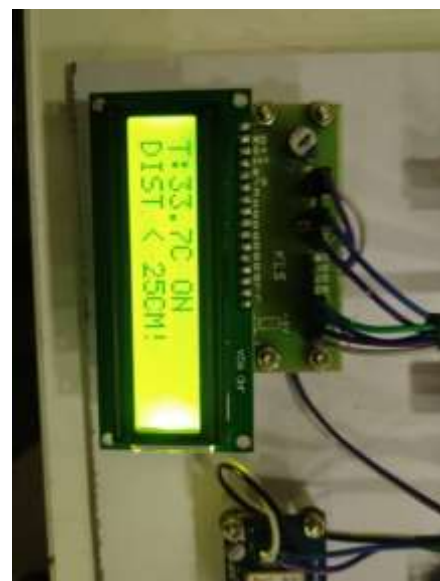
Fig5- LCD-Based Real-Time Temperature and Distance Monitoring System
