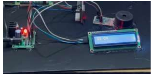
Fig. 12. Ultrasonic sensor distance output shown on LCD module
