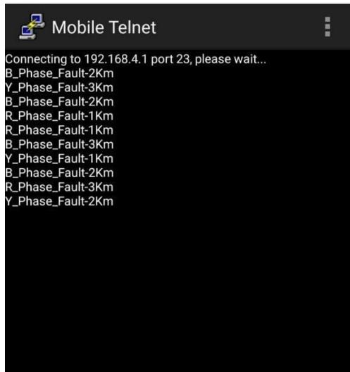
Fig. 6. Mobile telnet showing fault distance
