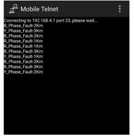
Fig. 6. Mobile telnet showing fault distance
