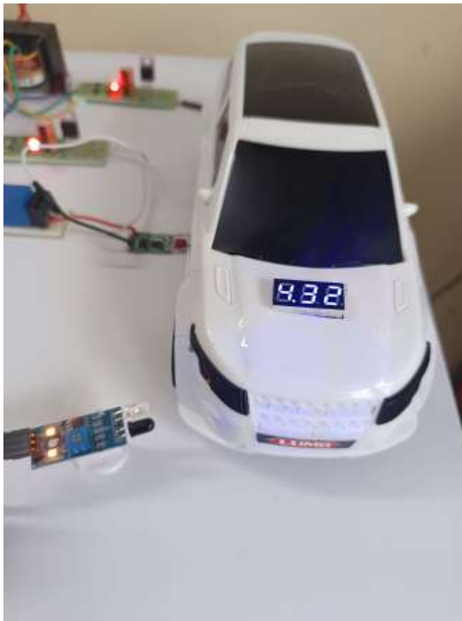
Figure 5. IR Sensor Car Detects And Car Charging Shows In Display
