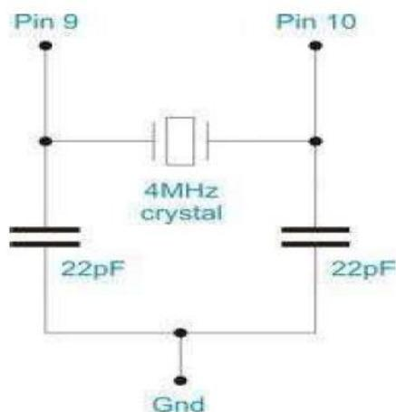
XTAL1 and XTAL2 are input and output, respectively, of an inverting amplifier which can Crystal or a ceramic resonator may be used. The CKOPT Fuse selects between two different Oscillator amplifier modes. When CKOPT is programmed, the Oscillator output will oscillate a full rail-to-rail swing on the output. This mode is suitable when operating in a very noisy environment or when the output from XTAL2 drives a second clock
