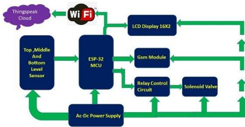
Figure 5. IoT-Driven Infusion Monitoring & Management System Block Diagram & Process
