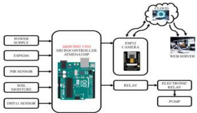
Figure 5.1 Block Diagram
