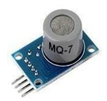
In the proposed project a gas sensor called MQ7 is used, the MQ7 is a simple-to-use Carbon Monoxide (CO) sensor suitable for sensing CO concentrations in the air. It can detect CO-gas concentrations anywhere from 20 to 2000ppm. MQ7 is a high sensitivity to carbon monoxide and stable and long-life span.
