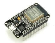
ESP32 is a series of low-cost, low-power system on chip microcontrollers with integrated Wi-Fi and dual-mode Bluetooth. The ESP32 series employs a TensilicaXtensa LX6 microprocessor in both dual-core and single-core variations and includes built-in antenna switches, RF balun, power amplifier, low-noise receive amplifier, filters, and power-management modules. ESP32 is created and developed by Espressif Systems, a Shanghai-based Chinese company, and is manufactured
