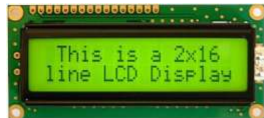
Fig 4. I2C LCD Display
