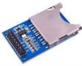
Fig 6: SD Card Module
