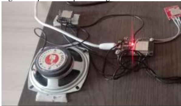
Figure 6. Speaker Output Testing for Audio Alerts
