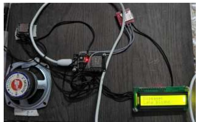
Figure 10. LED Display Showing Detected Leaf Disease
