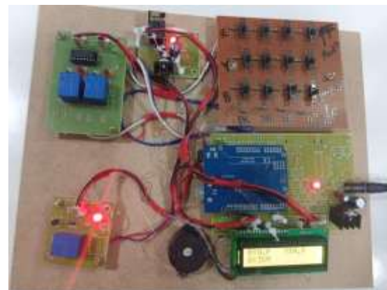
Fig. 5. LCD output and system response during fault condition.
