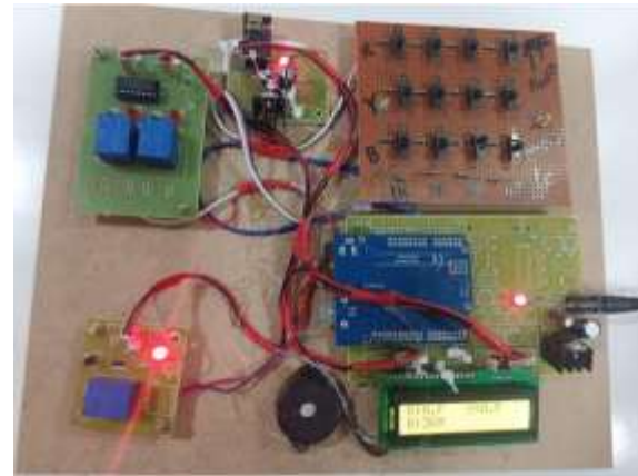
Fig. 4. LCD output and system response during fault condition.
