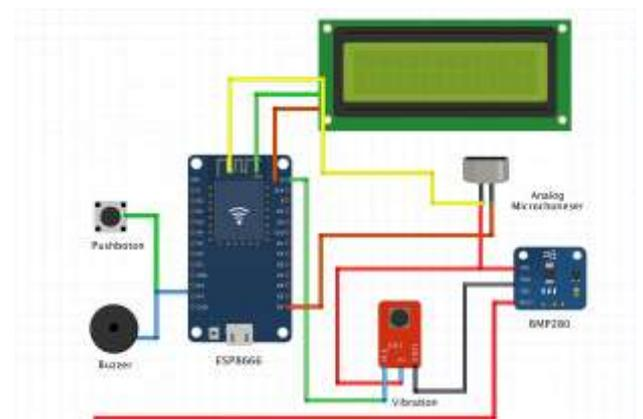
Fig. 2. Inhaler Unit Side Circuit Connections
