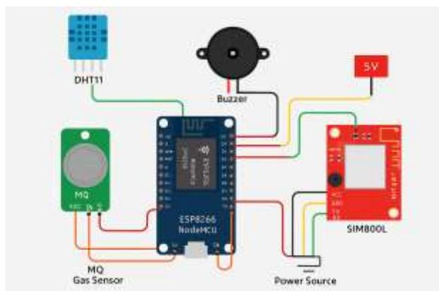
Fig. 3. Band Unit Side Circuit Connections
