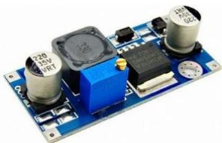
**Fig -5:** DC to DC Buck Converter
