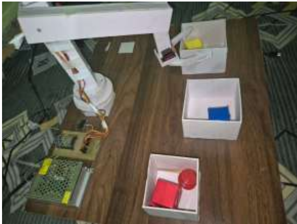
Fig. 3: Color-Based Object Segregation Using Vision-Guided Robotic Arm System
