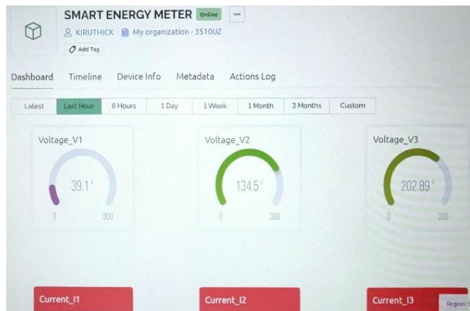
Fig -6: Blynk dashboard displaying real-time data.
