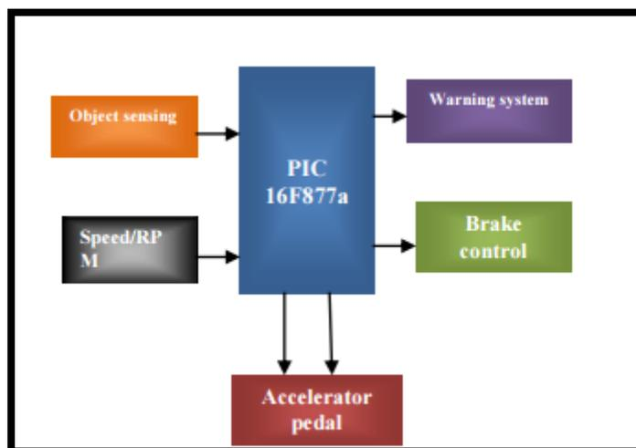
In the Figure, the object sensed using any of the object sensor is given as input along with speed obtained from the RPM counter which will be sent to the controller based on the commands provided it will calculate the speed that's need to be controlled based on the PID algorithm
