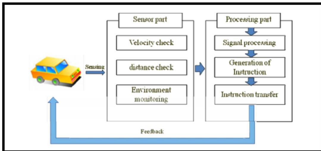
The auto-braking system was designed by VHDL and fabricated using FPGA to prevent accident. The system was mounted on a miniature car and tested. When the distance was getting closer, the auto-braking system was working and the speed will slow down if a driver does not reduce the speed of automobile. We also fabricated the auto-braking system using LabVIEW. We will replace an ultrasonic sensor with a radar sensor as the auto-braking system is mounted on a real automobile.
