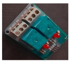
Figure 2 Relay Module
