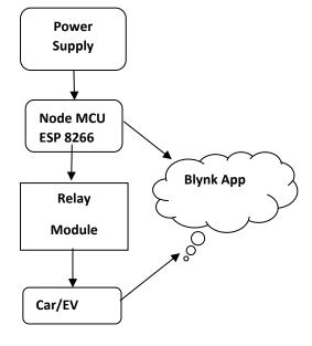
Figure 3 Block Diagram of Proposed System
