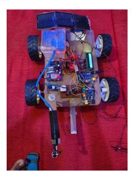
suspicious regions. GSM sound tracker, GPS tracker, smart cellphones plus advanced applications and RC truck equipment were brought together to do three main tasks for metal landmines, a) Tracing,-b) Detecting,-c) pinpoint location coordinates.
