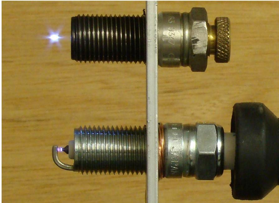
Top – Laser Ignition system, Bottom – Spark Plug Ignition system
