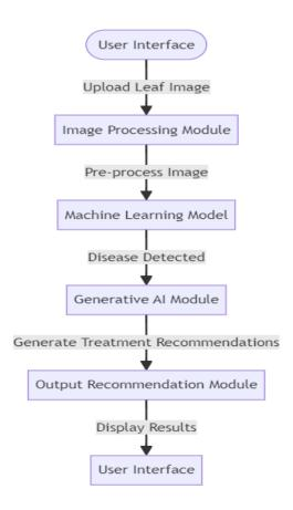
The architecture of the Leaf Doctor system forms the foundational structure that enables accurate and real-time plant disease detection. It outlines the interaction between the user interface, image processing pipeline, and AI-based classification engine.
