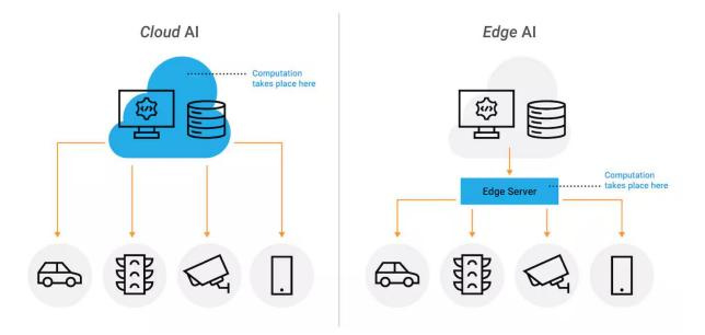
Fig. 3 Comparison of Cloud AI and Edge AI. Adapted from [6]
