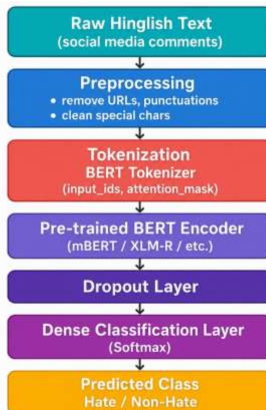
Figure 1. Illustration of End-to-end architecture of the Hinglish hate speech detection model showing preprocessing, tokenization, BERT encoding, and classification.
