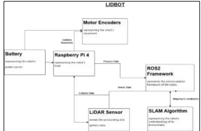
Figure 1: Block Diagram of LiDBot
