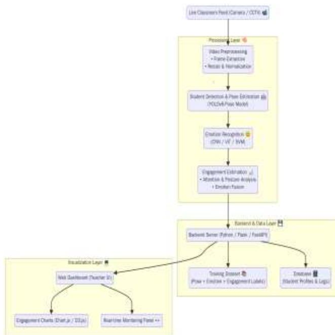
The proposed system is designed as a **real-time intelligent classroom monitoring framework** that integrates computer vision, deep learning, and behavioral analytics to recognize students and evaluate their engagement. The architecture is modular, scalable, and optimized for live classroom environments where multiple students must be tracked simultaneously.
