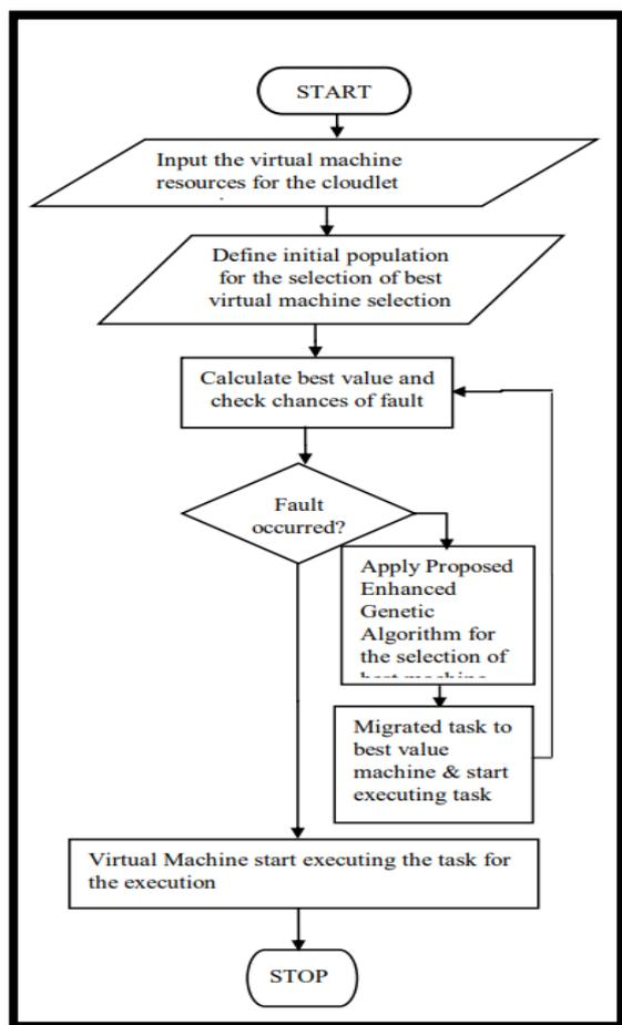
Fig 1.1 FLOWCHART OF IMPROVED GENETIC ALGORITHM
