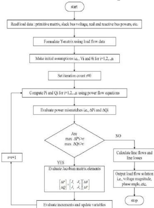
Fig 1).Detailed flowchart of Newton Raphson method
