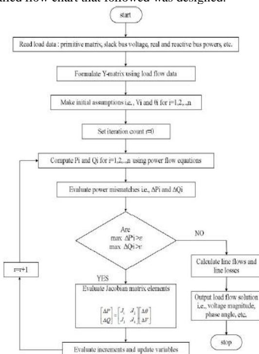
Fig 1).Detailed flowchart of Newton Raphson method
