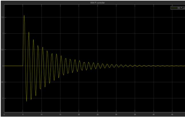
Fig 3 Change in frequency ( $\Delta f$ ) response for PI controller.
