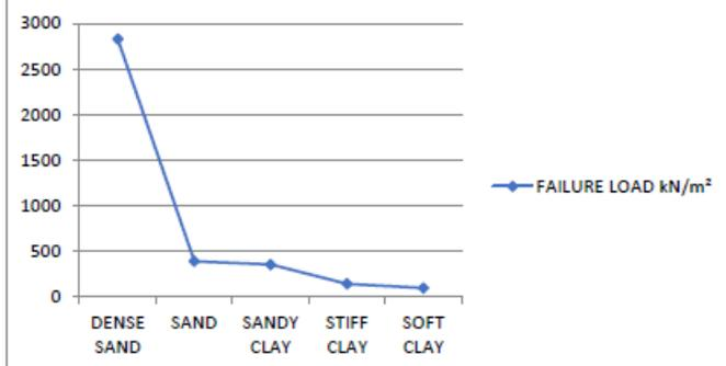
**Figure 1.4:** Failure load intensity graph for dense sand, sand, sandy clay, stiff clay and soft clay under axial load
