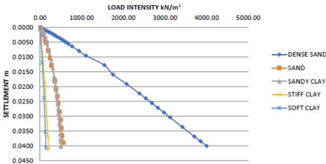
**Figure 1.3:** Load-Displacement curve for dense sand, sand, sandy clay, stiff clay and soft clay under axial load.
