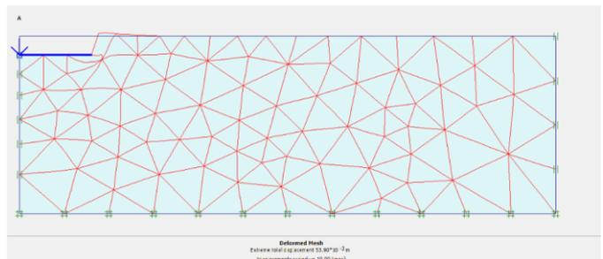
**Figure 1.7:** Mesh deformation for sandy clay having settlement of 57 mm
