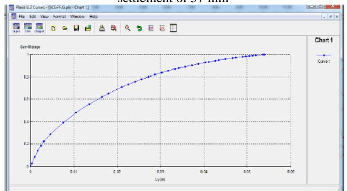
**Figure 1.8:** Load-Displacement curve obtained for Sandy Clay
