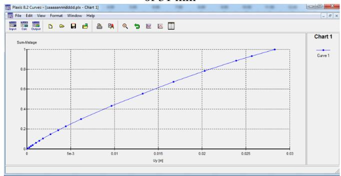
**Figure 1.6:** Load-displacement curve obtained for sandy soil
