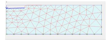
Figure 1.5: Mesh deformation for sandy soil having settlement of 31 mm
