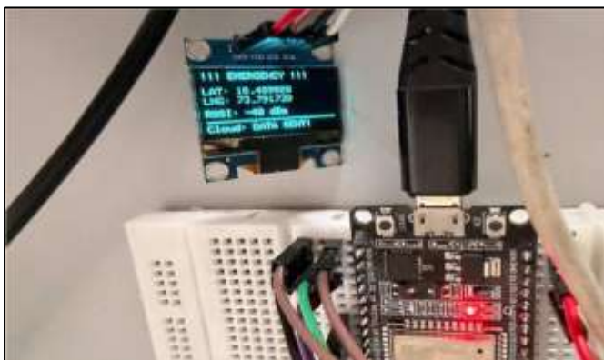
Fig -4: Transmitted location with coordinates and signal strength
