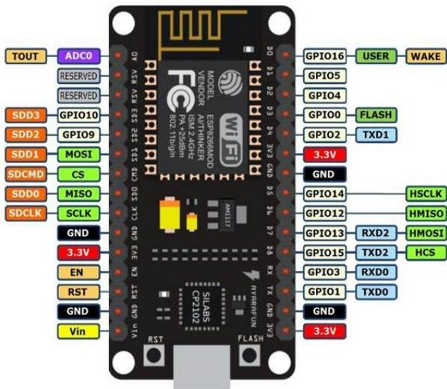
Fig.4 Pin Diagram of Node MCU
