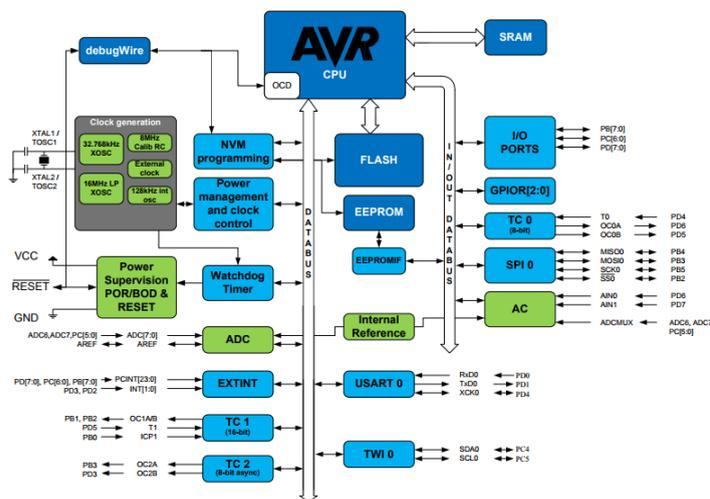
Analog comparator: On-chip analog comparator is available. An interrupt is assigned for different comparison result obtained from the inputs.
