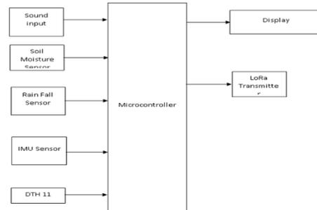
BLOCK DIAGRAM FOR LoRa TRANSMITTER
