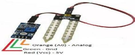
The readout from the probe is not linear with water content and is influenced by soil type and soil temperature. In This sensor we are using 2 Probes to be dipped into the Soil. As per Moisture We will get Analog Output variations from 0.60volts - 5volts. Input Voltage 5V DC.
