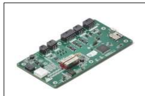
Fig: Battery Management System (BMS)
