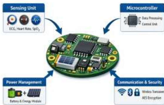
Fig. 3. Components of a Wearable Sensor Node
