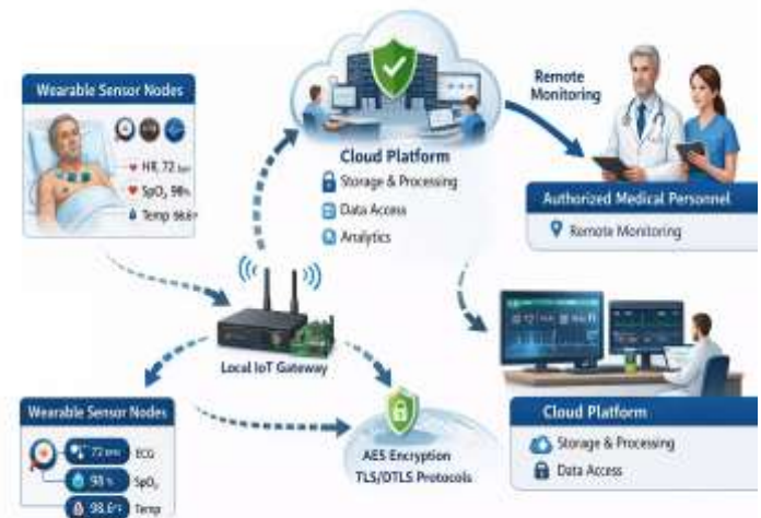
Fig. 1. General Architecture of the IoT-Based Remote Healthcare Monitoring System
