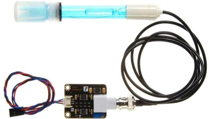
A pH sensor is essential for measuring the acidity or alkalinity of a solution accurately. Typically operating at 5V DC, it consumes minimal power, suitable for various applications, including those powered by batteries. Power is provided through the
