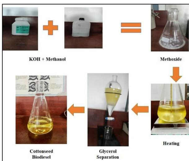
**Figure 3: Transesterification process of Cotton Seed Biodiesel.**
