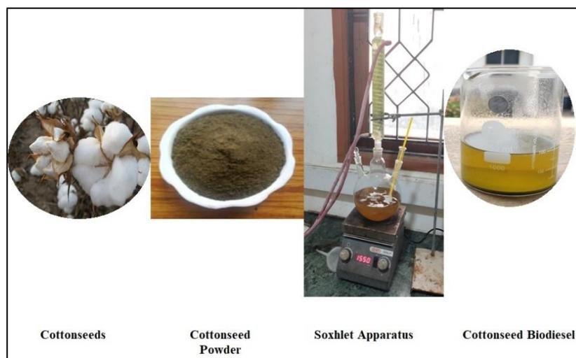
**Figure 2: Cotton Seed and Oil Extraction Process**
