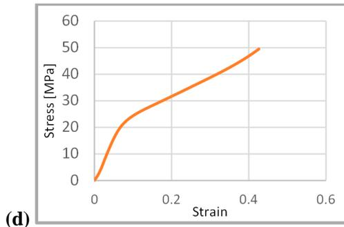
**Figure no.4 Results of brick sample 1** (a) Compression strength values of brick plastic to sand 3:1 (b) Stress-strain curve with 0 g bitumen. (c) Stress-strain curve with 4.5 g bitumen. (d) Stress-strain curve with 13.5 g bitumen.
